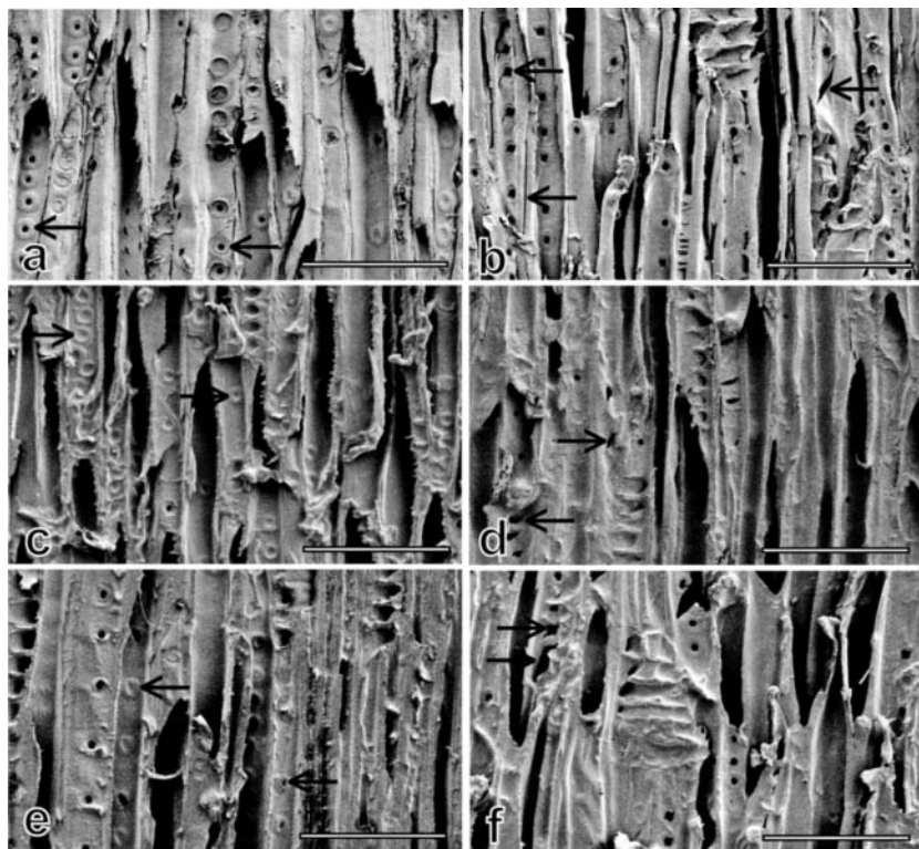
Figure 4. Scanning electron photomicrographs of the surfaces of untreated and treated veneers before and after exposure to 200 hours of accelerated weathering. Scale bars = 100 \mu\text{m} ; Fig. 4a = Unexposed control, note bordered pits (arrowed); Fig. 4b = Untreated exposed control, note micro-checking of bordered pits (arrowed top left and right) and separation of tracheids (arrowed bottom left); Fig. 4c = Unexposed veneer treated with HEPBP-Pa, note film obscuring bordered pits (arrowed); Fig. 4d = Veneer treated with HEPBP-Pa after accelerated weathering, note slight micro-checking of bordered pits (arrowed); Fig. 4e = Unexposed veneer treated with HEPBP, note film obscuring bordered pits (arrowed); Fig. 4f = Veneer treated with HEPBP after accelerated weathering, note slight micro-checking of bordered pits (arrowed); Fig. 4g = Unexposed veneer treated with UVA/HALS, note film obscuring bordered pits (arrowed); Fig. 4h = Veneer treated with UVA/HALS after accelerated weathering, note micro-checking of bordered pits (arrowed top right) and separation of tracheids (arrowed bottom); Fig. 4i = Unexposed chromium trioxide treated veneer, note cell wall checking (arrowed left); Fig. 4j = Chromium trioxide treated veneer exposed to accelerated weathering, note micro-checking of bordered pits (arrowed left). ( Continued )
